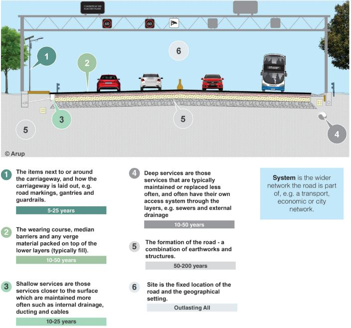
Figure 1 Layers-based approach for road assets
